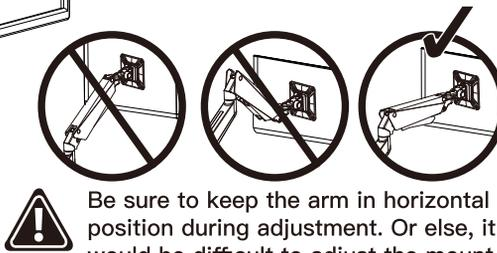
Be sure to keep the arm in horizontal position during adjustment. Or else, it would be difficult to adjust the mount.
